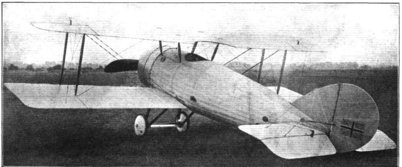
THE VICKERS E.S. 1, OR “BARNWELL BULLET.” —Note the stream-line body. The engine was a 100 h.p. Gnome monosoupape
